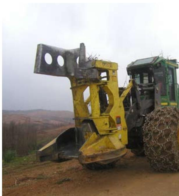
Fig. 12 – Cortador empilhador florestal *whelled feller-buncher*.
